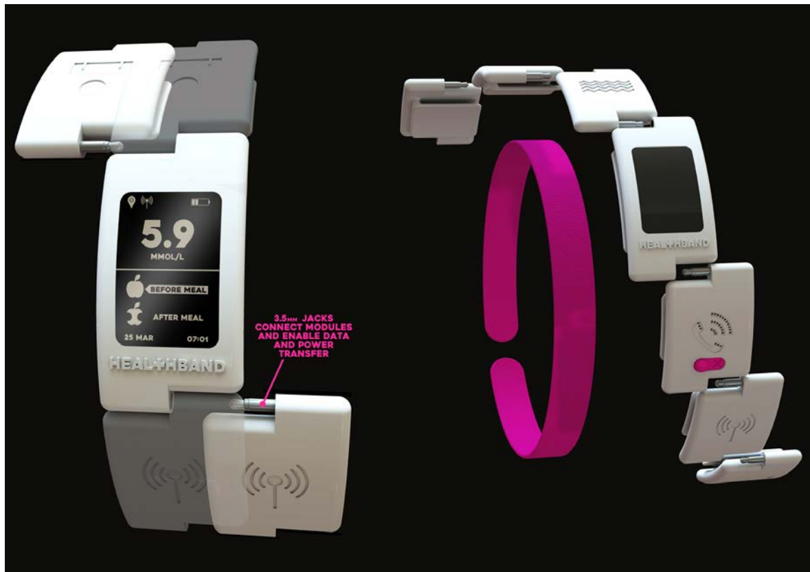
Figure 5. The HealthBand wearable’s design is modular and open source enabling different parties to improve existing modules and/or develop new ones with alternate functionality.
