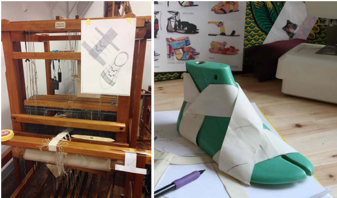
Figure 6. Examples of 3D non-digital design processes including paper modelling and sampling on a 6 shaft floor loom
