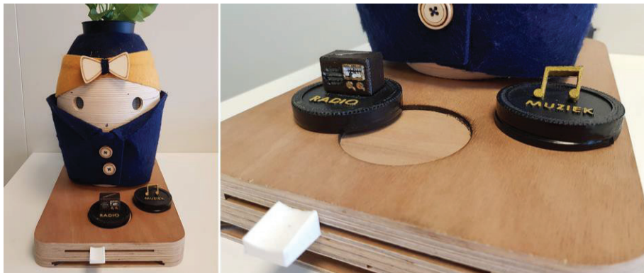
Figure 4 - Prototype for playing music. Placing a disc on the spot in the centre will start the corresponding music. The audio volume is controlled by the white slider positioned at the front.
