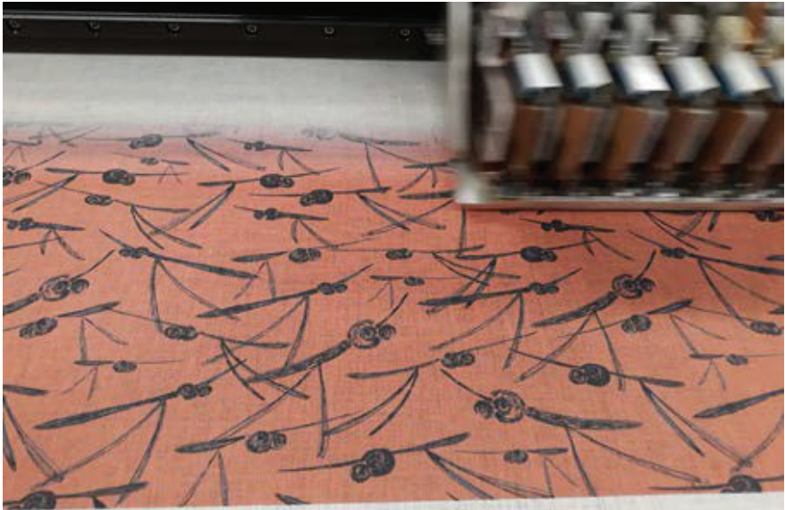
Figure 2. Experimenting with digital printing on textiles in Metropolia University of Applied Sciences. Textile prototypes are prepared e.g. by jacquard-weaving and digital printing techniques. Photo Ritva Jääskeläinen, pattern design Christa Eloranta.
