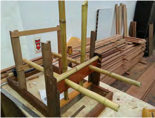
Figure 8. Gauge ready with the five rods positioned - prepared by author
