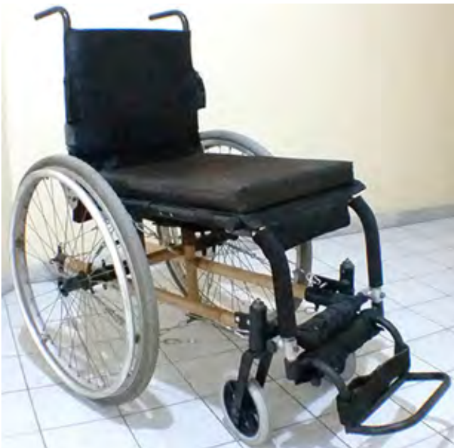
Figure 9. Test model of the wheelchair of tensegrity structure - prepared by author
