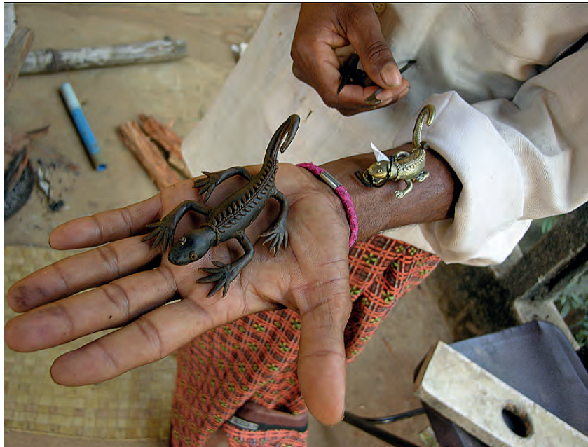
Figure 3. Dhokra or lost wax casting, photograph by the author.
