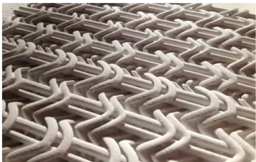
Figure 11: Unfired 3DP GLASS, open woven form
