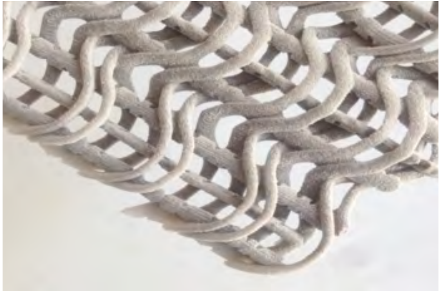
Figure 12: 3DP Fired glass, open woven form
