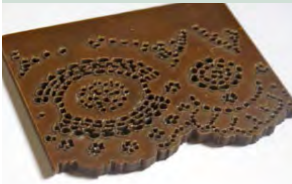
Figure 4: Flax reinforced bi-plastic, Faith Kane (2012)
