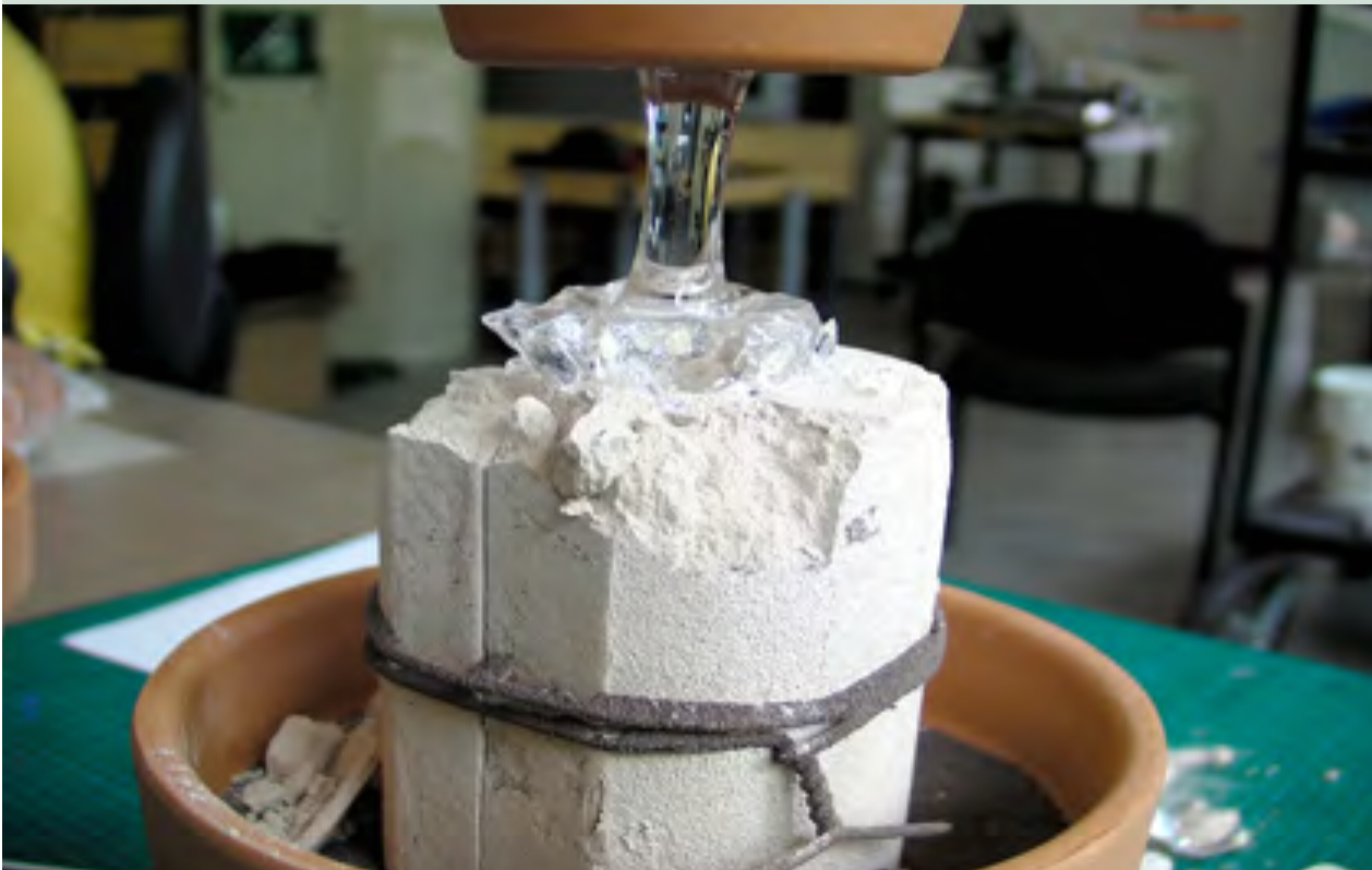
Figure 18: Glass casting setup, post-firing (form courtesy of Gayle Matthias, Senior Lecturer, Contemporary Crafts and Tavs Jorgensen, Research Fellow in 3D Digital Production, both of the Automatic Research Group at the University of Falmouth)
