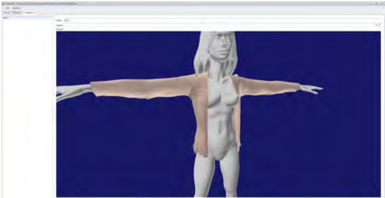
Figure 4: Screenshot of the simulation of a garment worn: tests of wearability, colour, working stitch, yarn quality.
