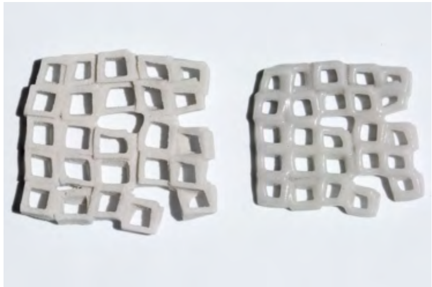
Figure 9: Loss of detail as transparency is achieved
