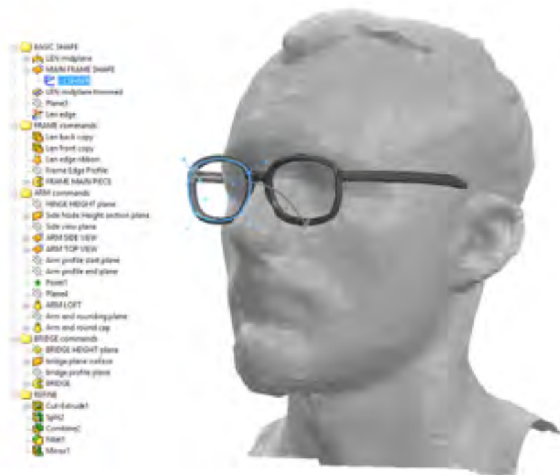
Image 1: SolidWorks model tree of the parametric eyeglasses frame
