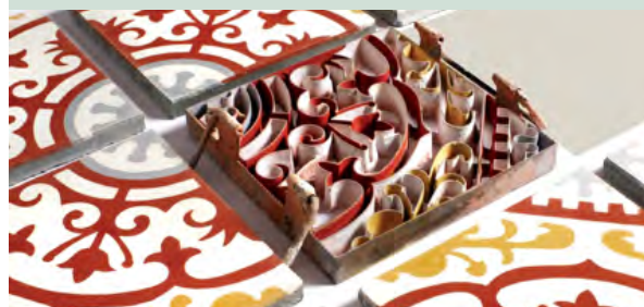
Figure 3: Encaustic Tile, elements of industrial production process (metal frame, finished tile)
