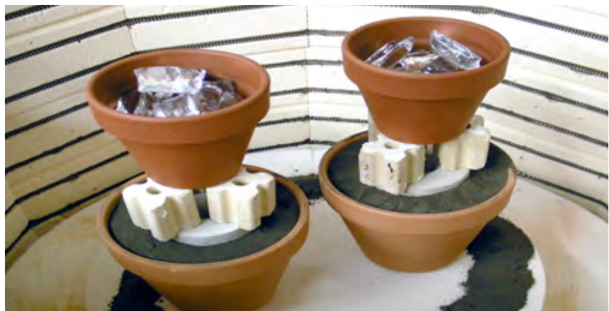
Figure 15: Glass casting setup, pre-firing (form courtesy of Gayle Matthias, Senior Lecturer, Contemporary Crafts and Tavs Jorgensen, Research Fellow in 3D Digital Production, both of the Automatic Research Group at the University of Falmouth)
