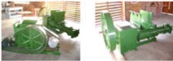
Figures 13 and 14 – Lamination equipment and vacuum extruder Source: Archive the Imaginary Laboratory
