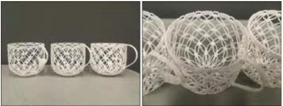
Figure 8. Printed cups in three different thicknesses: 0.8mm, 0.95mm, and 1.2mm.
