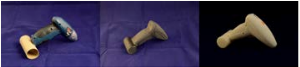
Figure 9 Mock-up, from model and 3D printed prototype - Desing by Jodean Steenkamp, photos by author
