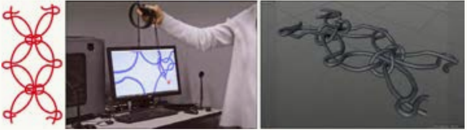
Figure 10. Drawing of a section of knots, crafting knots in VR, and CAD Model of a section of flexible knots.
