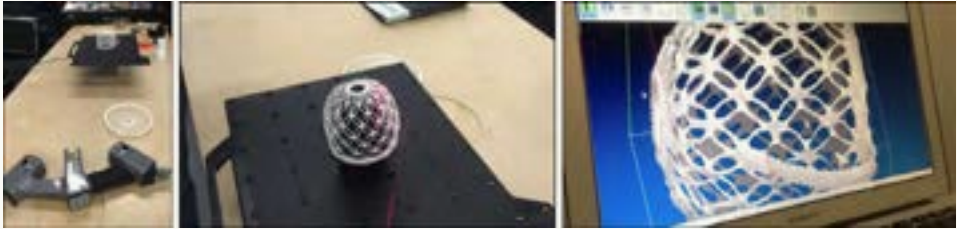
Figure 3. Polhemus Scorpion handheld 3d laser scanner; the scanning process; and the 3D scan.
