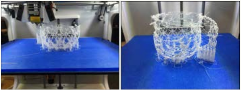
Figure 7. The first 3D printing of the cup on Tinkerine DittoPro 3D printer.
