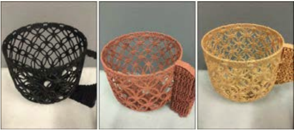
Figure 9. 3D printed cup using three different materials: (from left) PLA, copper, and wood.
