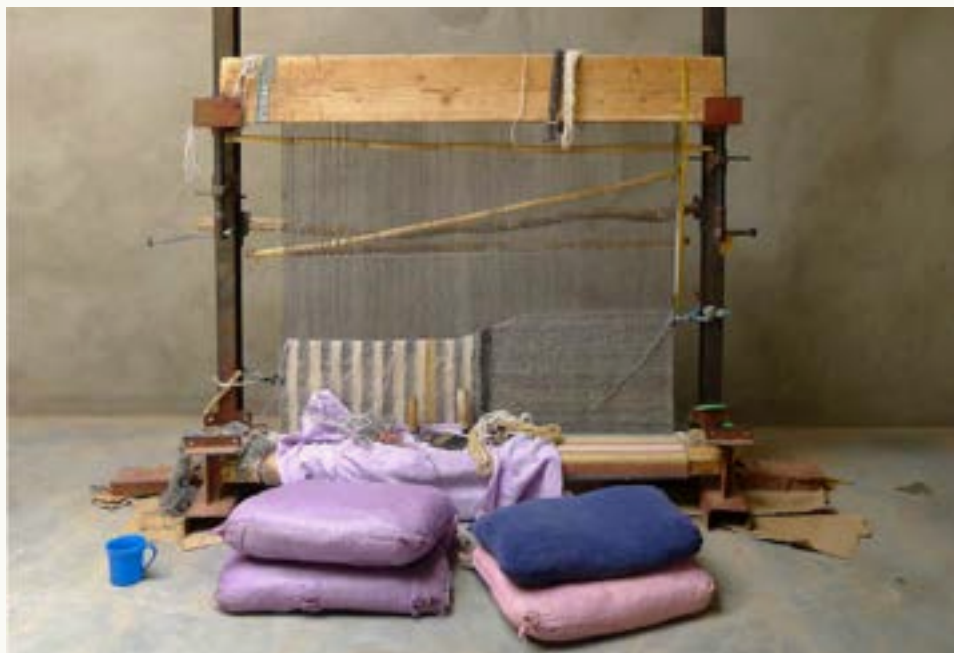
Figure 3. Vertical set-up of a weaving loom for the production of hand-woven carpets in Marokko. Picture credit: Salome Bäumlín, 2014
