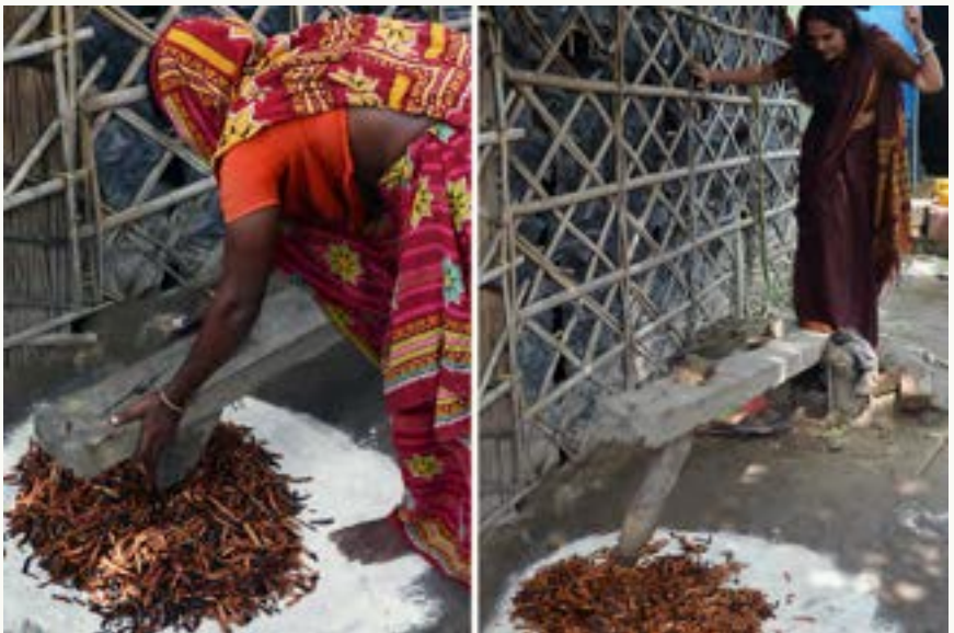
Figure 8. The “Dhenki”, an indigenous see-saw like wooden apparatus operated by legs to grind spices kept in the pit dug out on mud floor. The pit is lined with calcium hydroxide for dis-infecting the same (Photographs ©Indrajit De & Saumya Pande)
