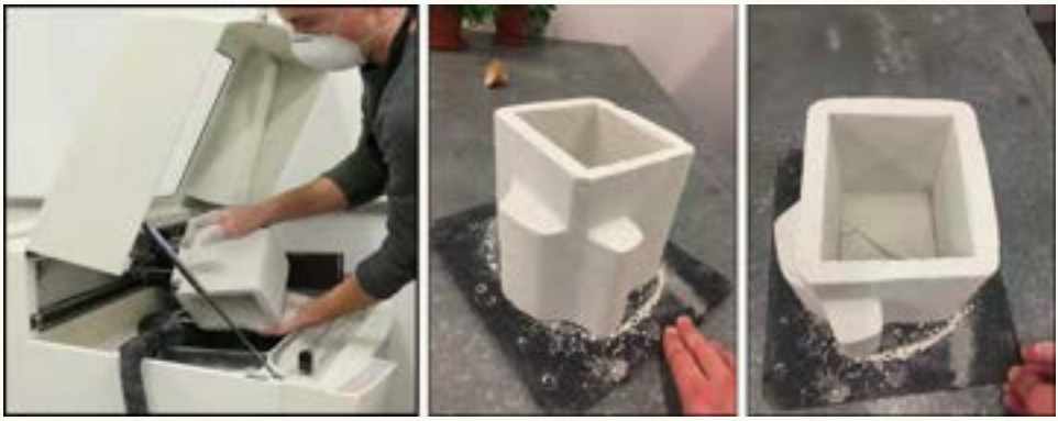
Figure 21. 3D printed moulds for glass casting, pre-firing.
