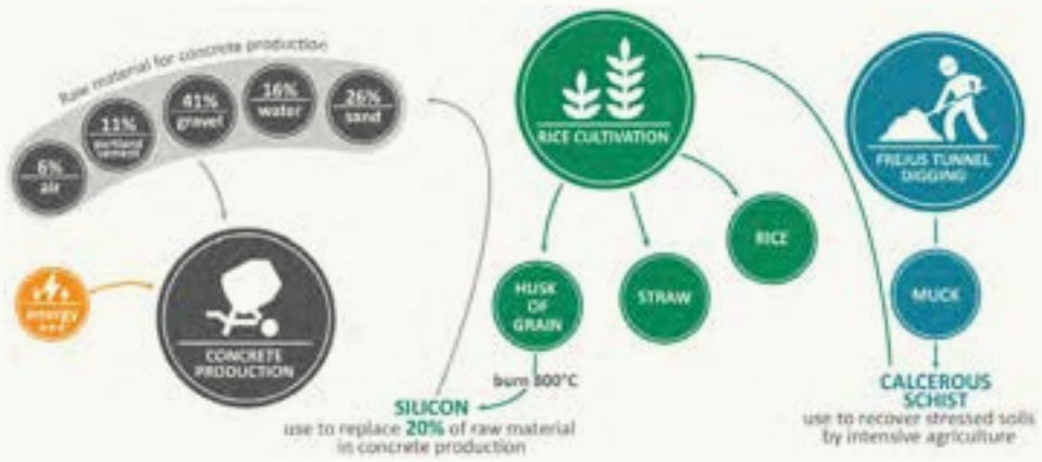
Figure 6. Application of Systemic Design approach in concrete production. 20% of concrete composition can be replaced by vegetable silicon obtained from rice husks (Chiaia, Fantili, Peruccio, 2017).
