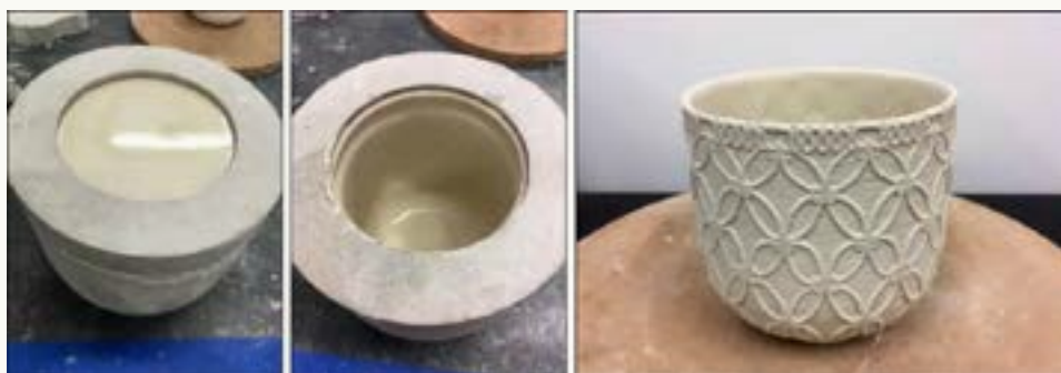
Figure 18. Slip casting porcelain using the 3D printed mould.
