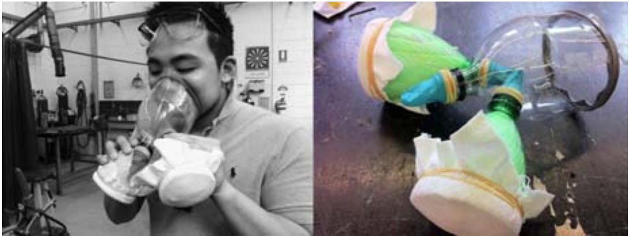
Figure 3 Example (b) Testing the DIY facemask for Indian Artisans 2011, by Lucas Chan, year 3 Product Design Engineering. This concept was inspired by two key ideas, the fact that India is one of the largest recyclers of plastic bottles in the world and secondly that Artisans are skilled at making things. The face mask is a low cost solution made from readily available material, plastic bottles, cotton fabric, elastic bands and rubber gloves that can offer significant health benefits to wood workers by providing a particle filtering face mask. This concept went through several iterations of Ideate and Prototype until a working prototype was resolved.
