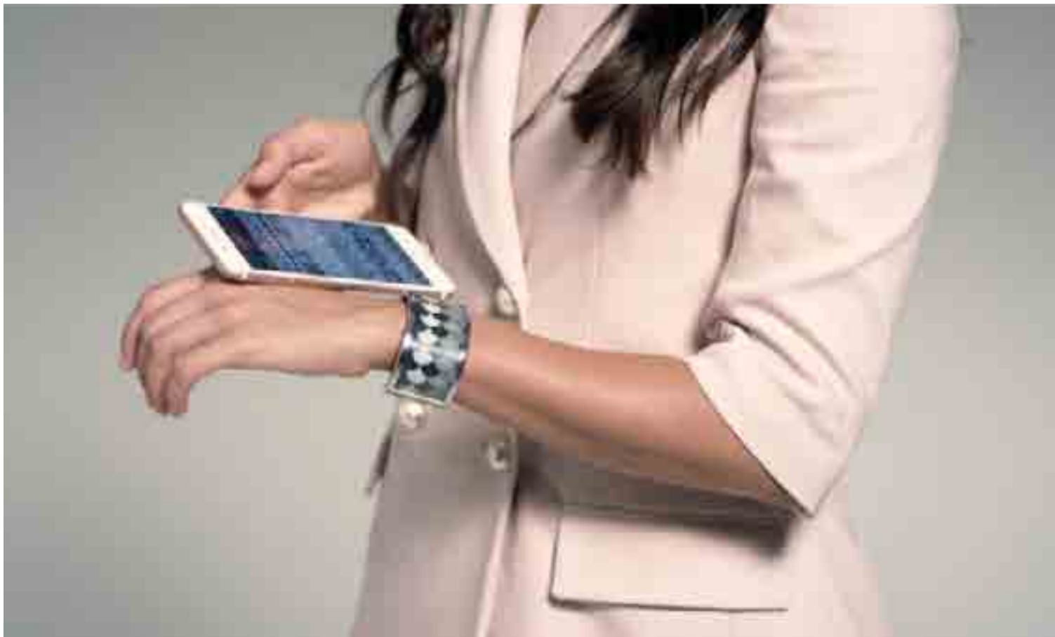
Figure 20.12: Tago Arc bracelet by L!ber8 Technology, Massachusetts, US The ultra-thin curved screen displays the selected pattern on the mobile application.
