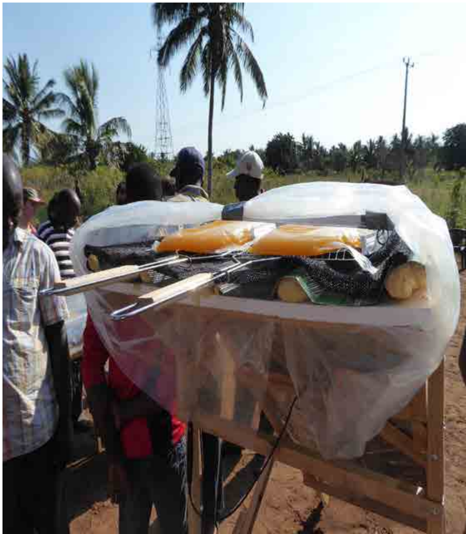
Fig 17.2: Preparation of the membrane bags, filled with juice. Personal photograph by author. 2017
