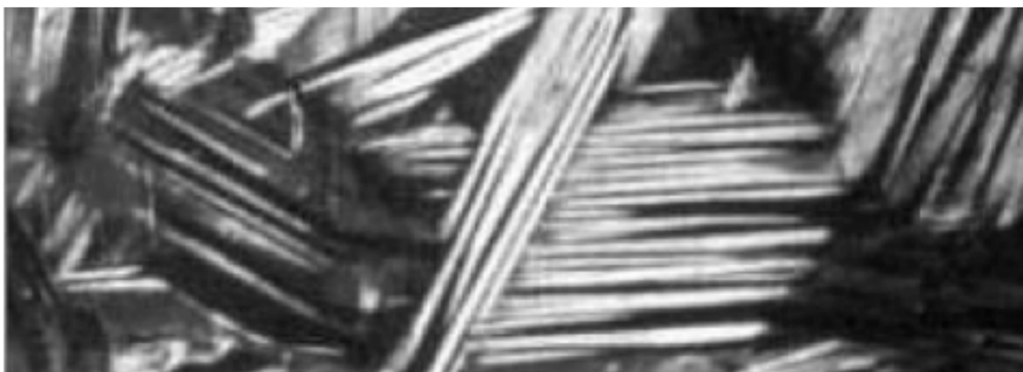
Figure 20.16: A highly magnified picture of the effect — an array of needle-shaped surface rumples that gives the spangle effect. Again, this material is only just being taken up by designers and manufacturers in a limited way. The jewelry design possibilities can be enhanced by selectively polishing away the spangle. Accessed October 29, 2017.
