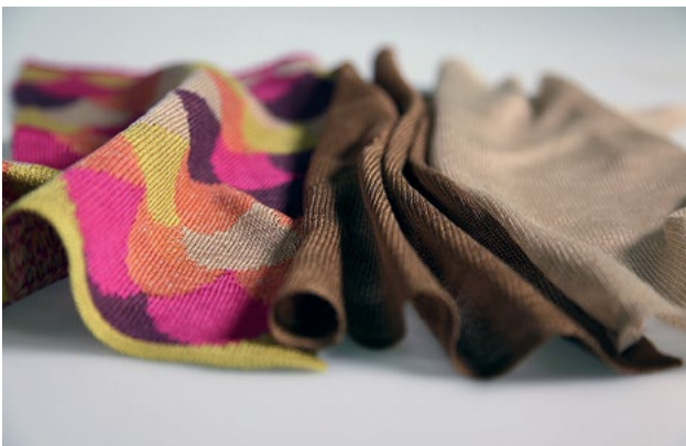
Figure 6.12. Cardboard and paper recycled into textiles by Ioncell-F technology, designed by Marjaana Tanttu in collaboration with Aalto CHEM (DWoC research project, 2014). Photograph: Eeva Suorlahti.
