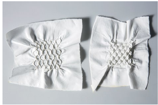
Figure 6.11. 3D structures of cellulose printed on cellulose by Pauliina Varis and Ilona Damski in collaboration with VTT (DWoC research project, 2016). Photograph: Eeva Suorlahti.
