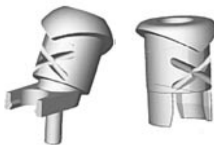
Figure 7. Two examples of measuring interfaces, designed by Dr Bjørn Iversen and Steinar Killi. The rounded top should fit in to the pelvis cup and will vary for different cup sizes. The cross on the middle is used for positioning the hip prosthesis (30 degrees angle) At the bottom we see the different ways to mount the interface to the prosthesis. To cover all possibilities the number of these parts will exceed 1000.
