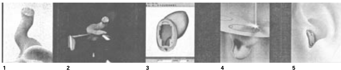
Figure 3. Work sequence for producing customised hearing aid.
